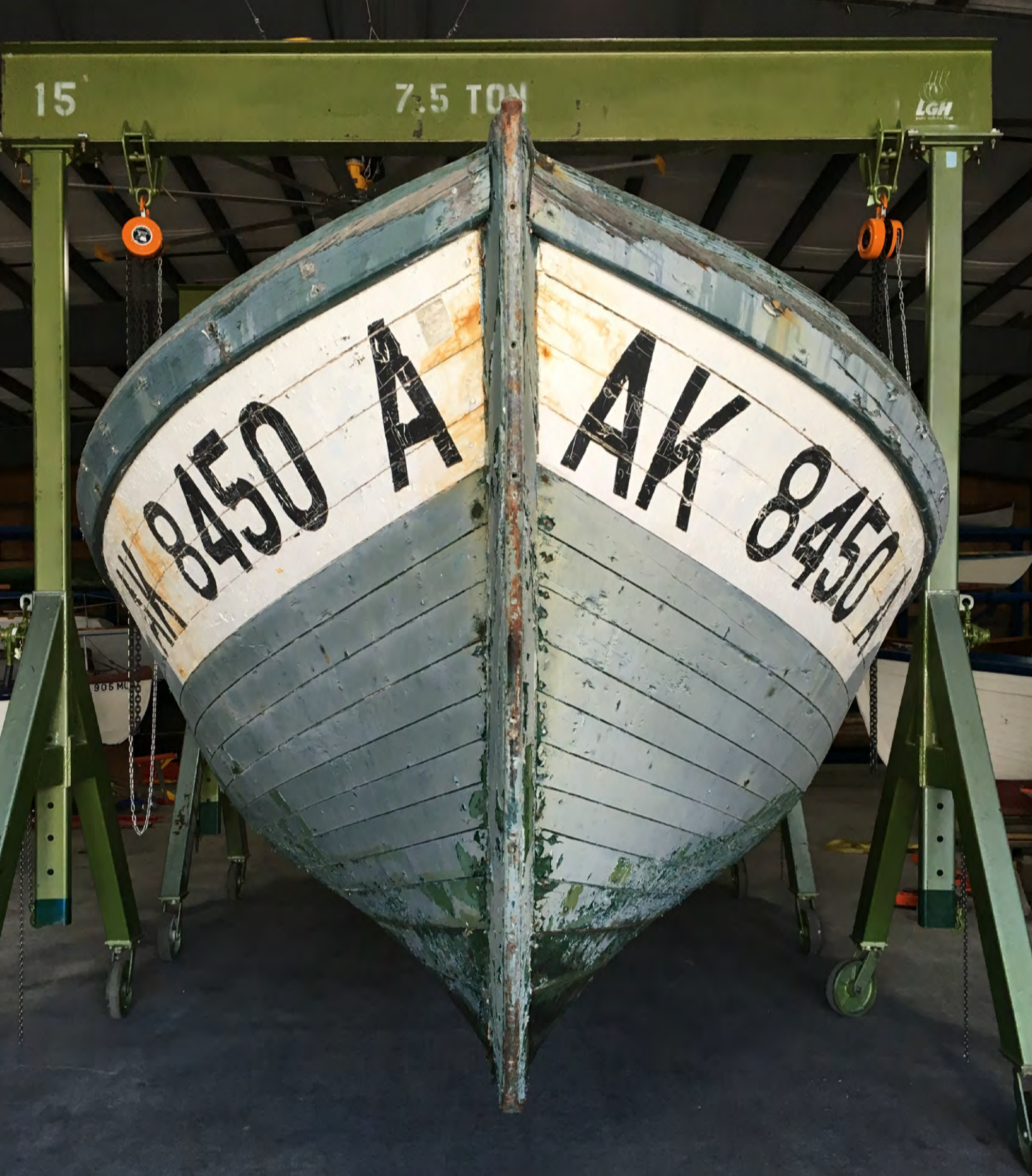
Bumble Bee Seafood's Alaska Gillnetter is lifted by the gantry crane to allow a new custom cradle to be built for her.
