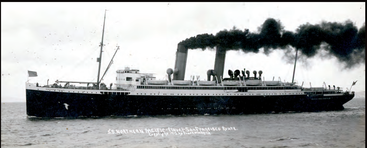
The Great Northern's identical sister ship, the Northern Pacific , is seen on her Flavel to San Francisco route. Each ship was 525 feet long, had a breadth of 63 feet, five decks, passenger capacity of 800 and crew of 200. The two smoke stacks were each 112 feet high. CRMM 411-16662
